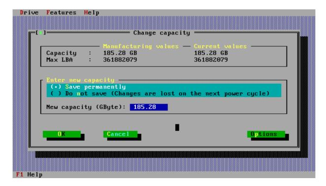
Some of the older Motherboards BIOS's don't support the larger capacity ATA drives, which are now available. The **Options** button provides a quick means of changing the drive capacity to just below the known boundary limits of 8GB, 32GB and 128GB, it also provides a quick means of resetting the drive to its maximum capacity.
