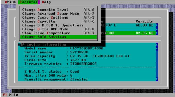
From the pull-down menu select the drive feature to be modified, for more detail on how to change each feature select from the links below.
