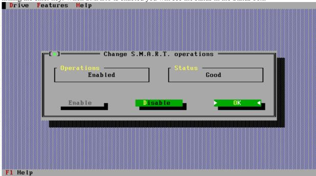
Note: on some system if SMART monitoring is enabled in the system BIOS then disabling SMART with this utility will be effective only until the next re-boot.
