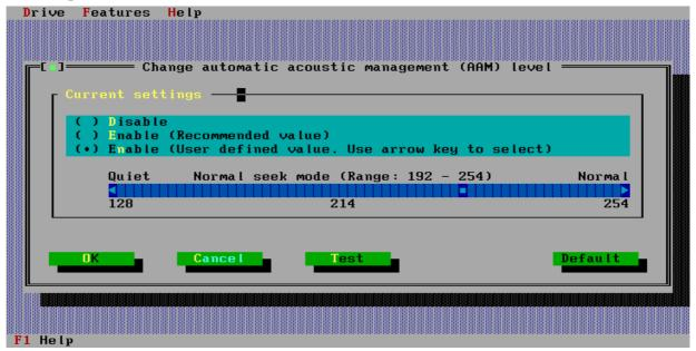
The **Test** option allows you to assess the effect changing the automatic acoustic management level will have prior to making the change permanent. To use this option select Test (Alt + T) or tab to the Test button and press enter. The following screen will be displayed.
