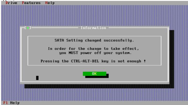
Once the Feature Tool has declared the operation to be successful, one must power cycle the drive. This must be achieved by a complete system shutdown and switched back on again.
