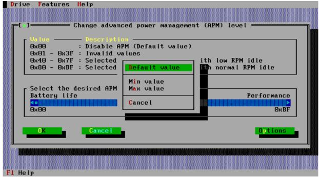
If the selected disk drive does not have or support changing the advance power mode then when this option is selected the following screen will be displayed.
